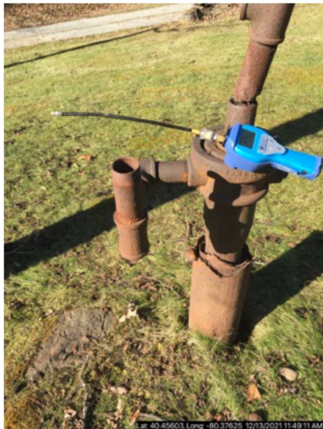
Figure 6. Photograph of SB Donaldson 2 with Bascom Turner EGA 411 4” above 2” production line venting gas at the wellhead. From PADEP (2021c)
