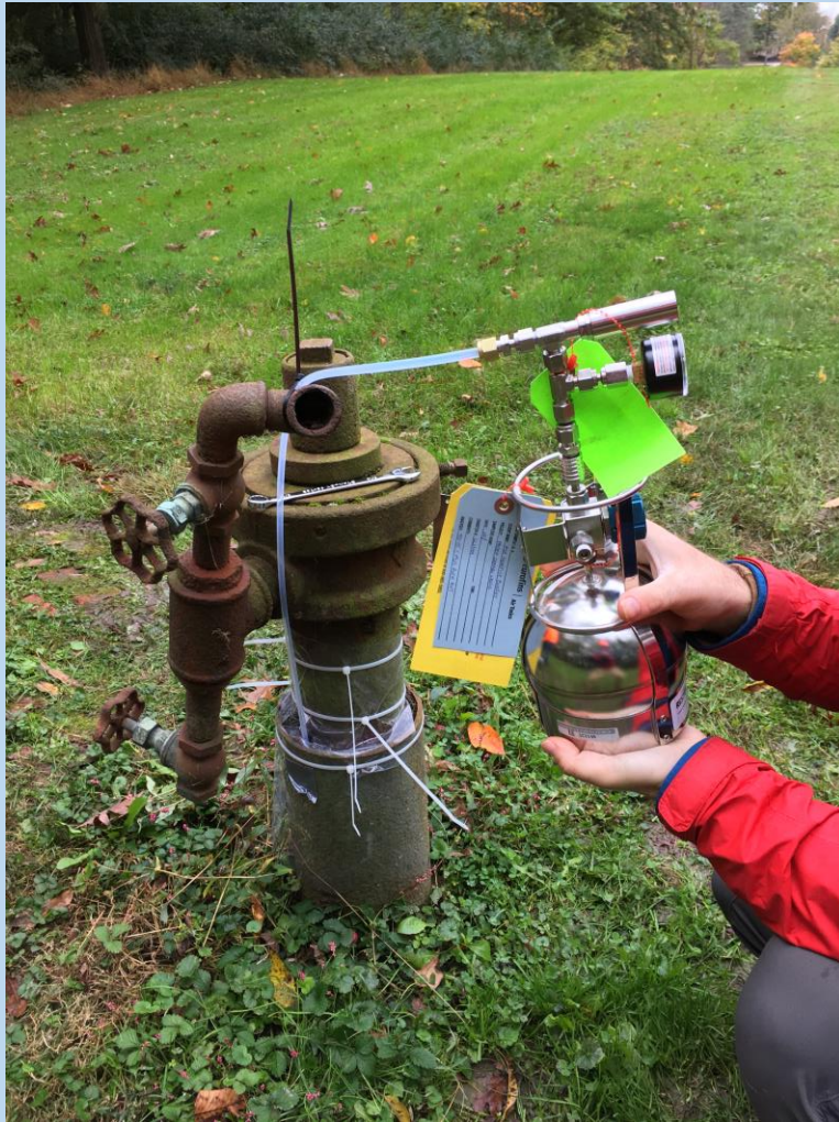
Photograph sampling abandoned well near house in western PA (DiGiulio)
